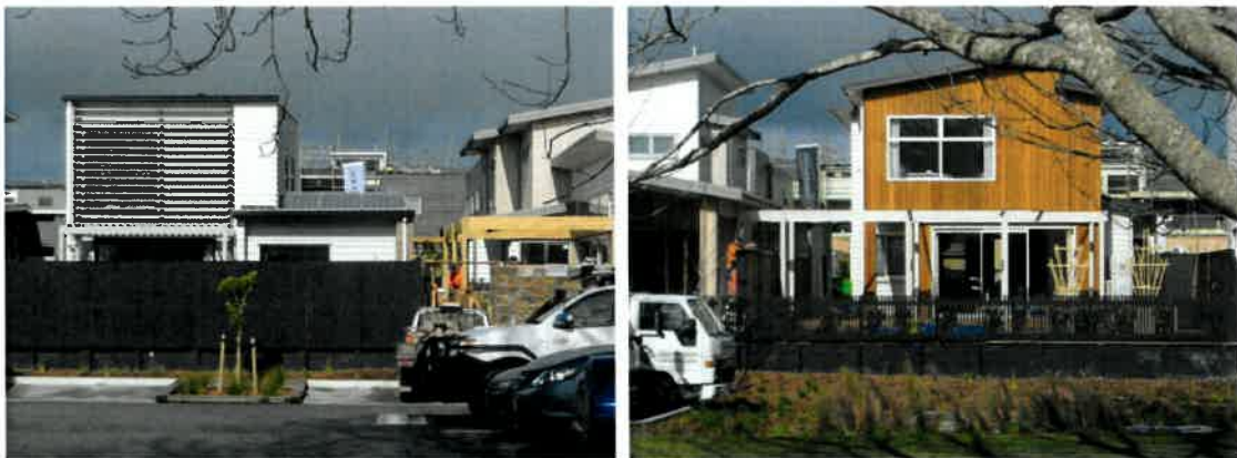
Figure 3: Example fence on left not accepted – does not provide passive surveillance or connection with the street.
